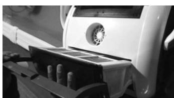
7. Skyv filterplaten tilbake i bassengroboten langs sporet
