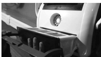
7. Slide the filter tray along the groove
