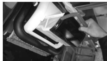
2. Lift the filter tray
